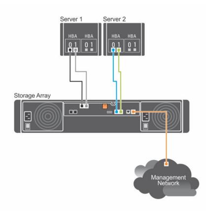
Figure 4. Two Hosts Connected to a Single RAID Controller Using One HBA
