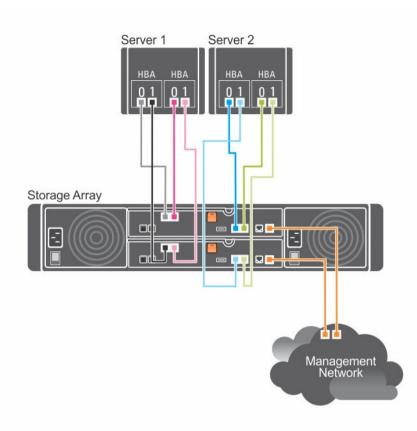
Figure 6. Two Hosts Connected to Two RAID Controllers
