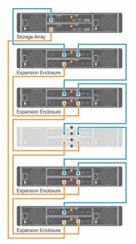
Figure 12. Single expansion cabling diagram
