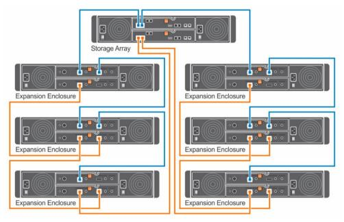
Figure 13. Dual expansion cabling diagram
