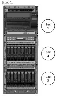
24 SFF hot-plug drive model: Tower – shown without the tower feet. 1 – 3 8 SFF SAS/SATA hot-pluggble HDD/SSD Cage Kit (s). 16 SFF hot-plug drive + 8 NVMe SSD model:
