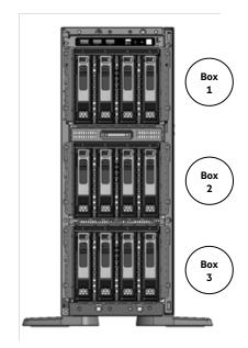
8 SFF hot-plug drive model: Tower – shown without the tower feet. 1 x 8 SFF SAS/SATA hot-pluggble HDD/SSD Cage Kit in Box 3. HDD Cage Blank in Box 2. Media Bay Blanks (2) and DVD blank (1) in Box 1.
