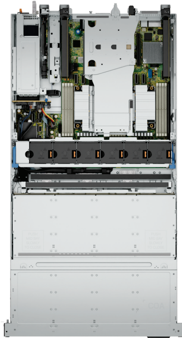
Figure 19. 3 x PCIe Low-Profile Slots + 2 x PCIe FH/FL Slots
