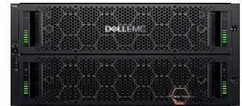
ME4084 SAN/DAS ARRAY (84 drive) 2.5" drive slots, 5U
